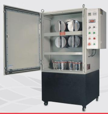
CPM machine is ideally suited for jewellery and other intricate components. The machine features a variable frequency drive for speed control and has replaceable polyurethane liners inside the barrels. This machine is compact and uses the latest technology in the transmission of rotary motion. The equipment can be supplied with stainless steel barrels for specific processes.
